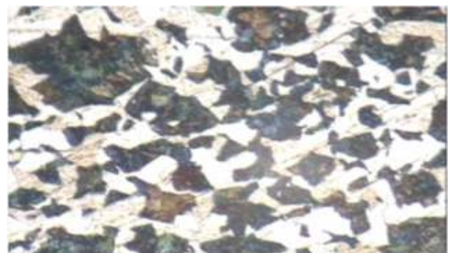
Fig-2: less pearlite microstructure of chain link
